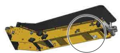
Fig 35 - Belt Scraper inside hopper frame
