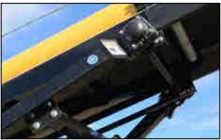
Fig 70 - Upper lift bearings
