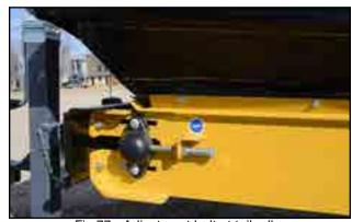
Fig 77 - Adjustment bolt at tail roller
