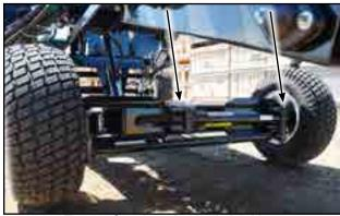
Fig 67 - Steering wheel axle bushings
