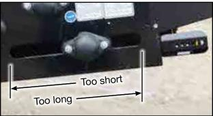
Fig 49 - "Slack Eliminator" roller. Belt length indication
