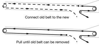
Fig 85 - Thread belt through conveyor
