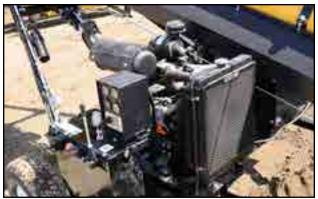
Fig 10 - Tier 4 diesel engine
