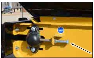
Fig 59 - Adjustment bolt on tail roller
