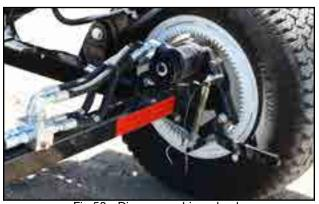
Fig 50 - Disengage drive wheels
