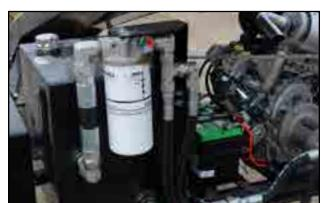
Fig 89 - Hydraulic Oil Filter
