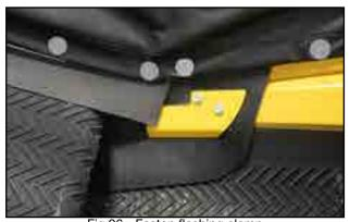
Fig 96 - Fasten flashing clamp
