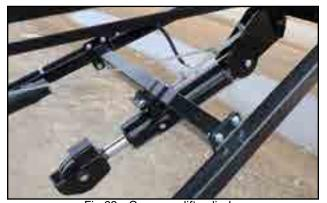
Fig 69 - Conveyor lift cylinder
