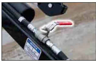
Fig 45 - Hydraulic valve to lift cylinder
