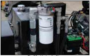
Fig 66 - Hydraulic filter
