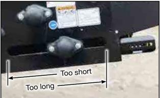
Fig 76 - "Slack Eliminator" roller. Belt length indication
