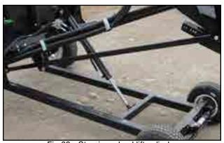
Fig 68 - Steering wheel lift cylinder
