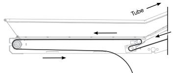
Fig 82 - Threading belt around hopper
