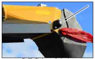
Fig 65 - Discharge roller bearing
