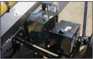
Fig 55 - Oil reservoir and fuel tank
