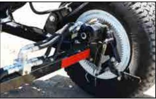
Fig 17 - Disengaged drive wheel
