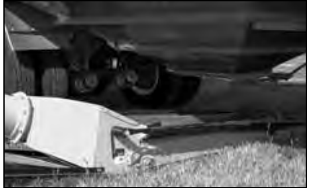
Fig 14 - Conveyor Under Truck
