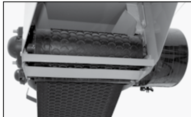
Fig 39 - Belt Aligned in Discharge Hood
