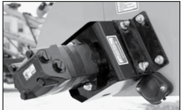
Fig 10 - Hydraulic Motor, Hoses not Attached
