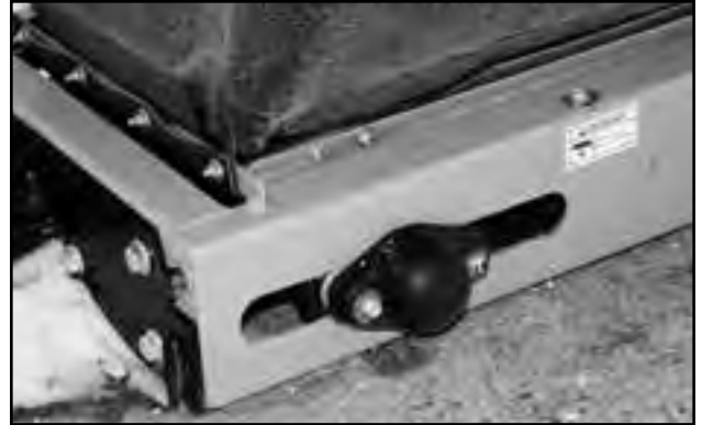
Fig 41 - Conveyor Belt Access Panel
