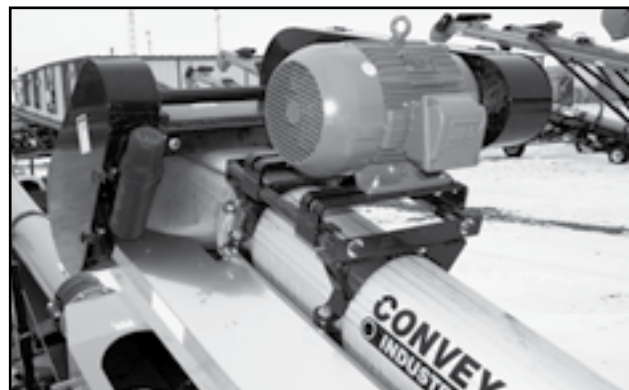
Fig 48 - Electric Motor, Speed Reduction Drive
