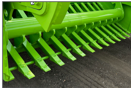
Replaceable teeth and 450 BHN Grate
