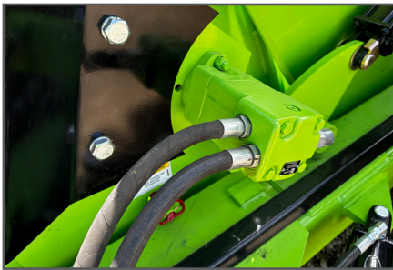
A hydraulic drive system provides a cushioned drive that can be easily reversed to free jammed rocks.
