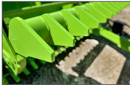
Batt tubing has 1/2" thick walls and wrap around, 5/8" 450 BHN hard-surfaced teeth. The heavy batt weight creates momentum reducing spring tripping
