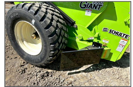
Standard 16.5L X 16.5 and even larger 560/45R22.5 tires offer superior flotation under heavy loads
