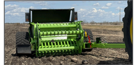
Large 3.5 cu.yd (2.68 cu m) hopper and extra wide 72" picking width
