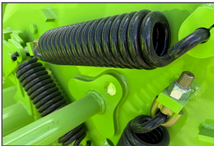
Extra heavy duty batt springs 450 BHN steel reel
