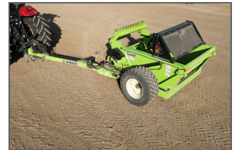
The longer, bent hitch pole improves operator visibility, from the cab window
