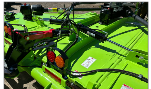
Hydraulic phasing cylinders replace turnbuckles and allow for parallel wing lift
