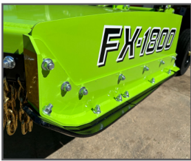
Replaceable, side bands and replaceable skid shoes
