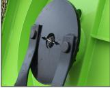
Heavy duty 3/4" thick blade disc with 4" blades and pentagon blade bolts
