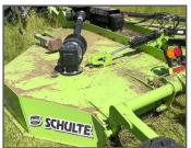
Continuously welded single domed deck
