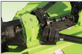
Forward mounted slip clutches
