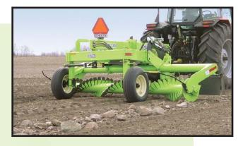
The SRW 1400 Pivoting Rock Windrower employs a side delivery frame arrangement which allows the operator to better control the size of windrows, regardless of rock conditions. The windrower's patented floating drum arrangement allows the wheels to be placed closer to the windrower drum, resulting in excellent ground following characteristics.
