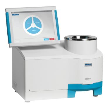
**Test Weight Module:** Can be equipped with a Test Weight Module that becomes an integrated part of the instrument.
