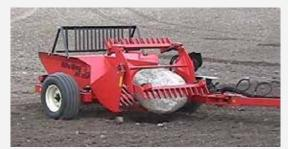
By positioning the rake and using the reels as a support, the RR250ST can pick rocks up to  $24" \times 45" (61 \times 144 \text{ cm})$  and the RR900ST picks rocks up to 28" x 55" (81 x 140 cm).
