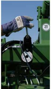
Single-point depth control allows the operating depth of the entire disc to be adjusted with a single setting. This simple adjustment, done at the front of the machine, is easy, safe, and precise. Single-point depth control is optional on all models.
