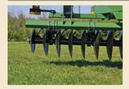
Wishek 812N-OCL Offset Disc features 28-inch (711 mm) blades on 11-inch (279 mm) spacing. The winged model comes with an OCL (Over Center Lock) system for complete leveling performance. The OCL system on the 812N unit prevents the disc wings from diving or lifting out of the ground by locking the wings rigid to the main frame.
