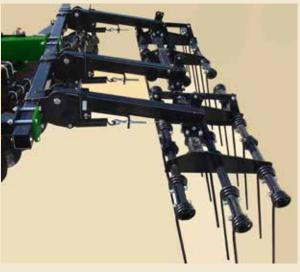
To assist in leveling the field and help create a better seedbed, add a 3-bar harrow. The tubular tooth bar harrow features  $\frac{5}{16}$  x 26-inch-long tines (16 x 660 mm) for strength and durability.
