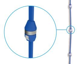
The OPI moisture cable has sensors placed on the cable commonly at 4' intervals in farm applications and 6' intervals in commercial applications. Moisture cables are used in grain depths up to 85'.
